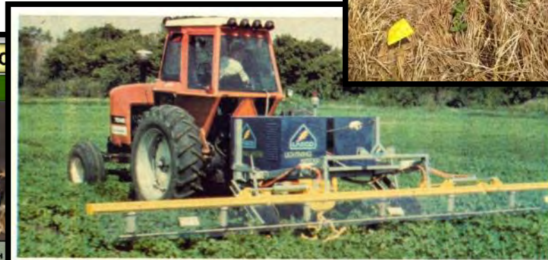
One end of machine's power circuit is electrically in contact with soil through a coulter. Other end of circuit is connected to boom which comes in direct contact with weeds growing taller than crop.
