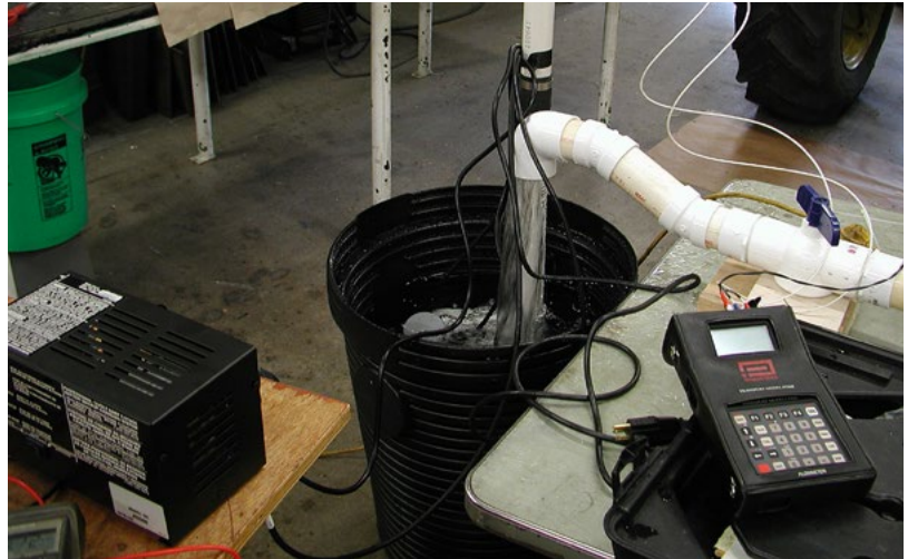
Figure 8. Backup pump test stand showing water flowing into sump that contains the two pumps. The charger is in the lower left and on the right is the ultrasonic flow meter used to measure the flow rate.
