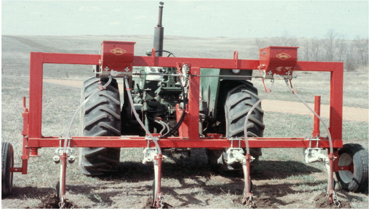
Fig. 1. Interseeding machine with two toolbars and four shanks.
