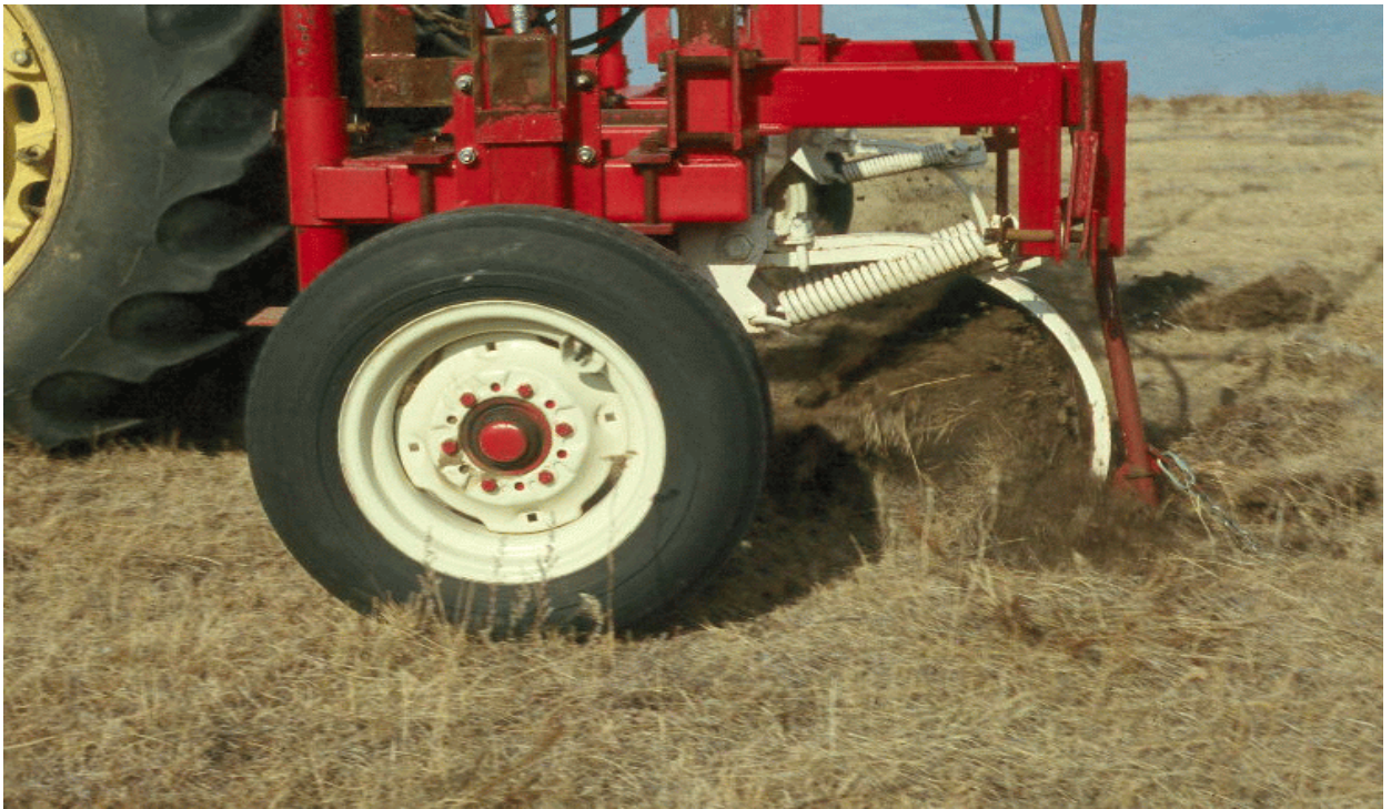
Fig. 4. Interseeding machine at ten-foot row spacings.
