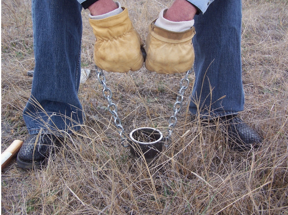
Figure 8. Capture cylinder is lifted by leg muscles with two hands on extractor chain handle.
