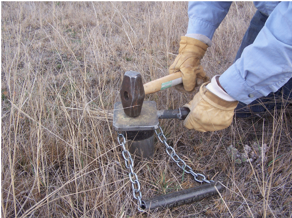
Figure 3. Striker plate set on top rim of capture cylinder is firmly struck with sledgehammer.
