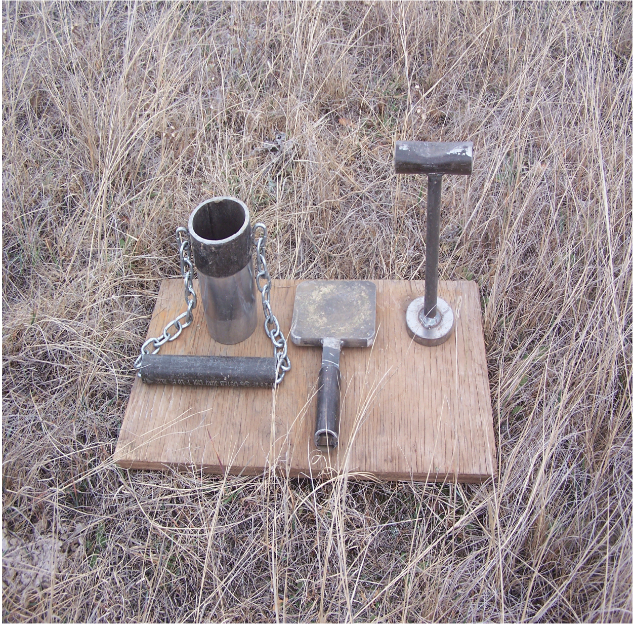
Figure 1. Three components of the humane soil beastie catcher: the capture cylinder with extractor chain, the striker plate, and the expulsion ram plunger.
