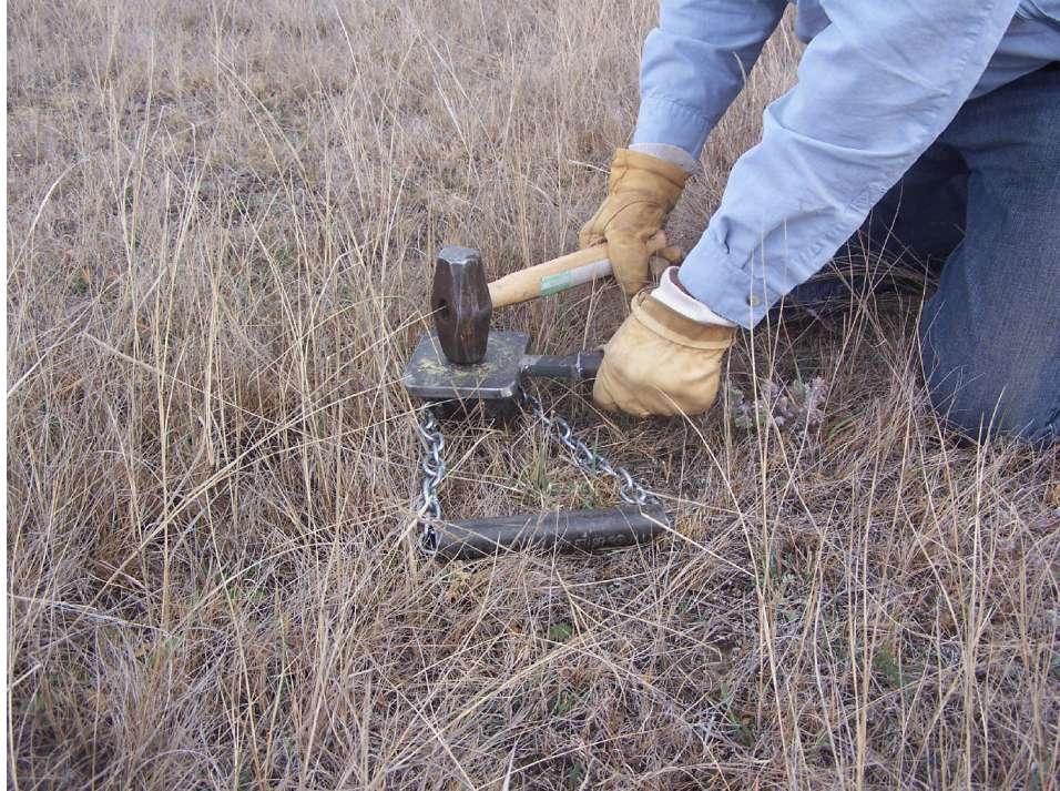
Figure 4. Repeated sledgehammer strikes drives capture chamber into the soil to the bottom of the cylinder collar.
