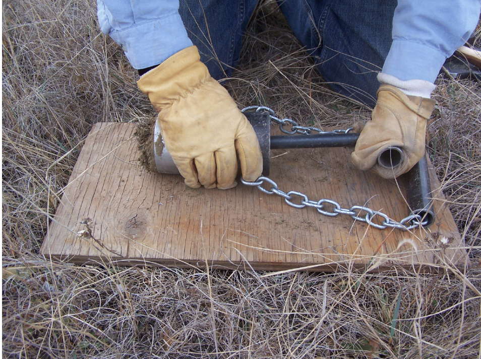
Figure 10. Expulsion ram plunger placed into top of capture cylinder laden with soil beasts.
