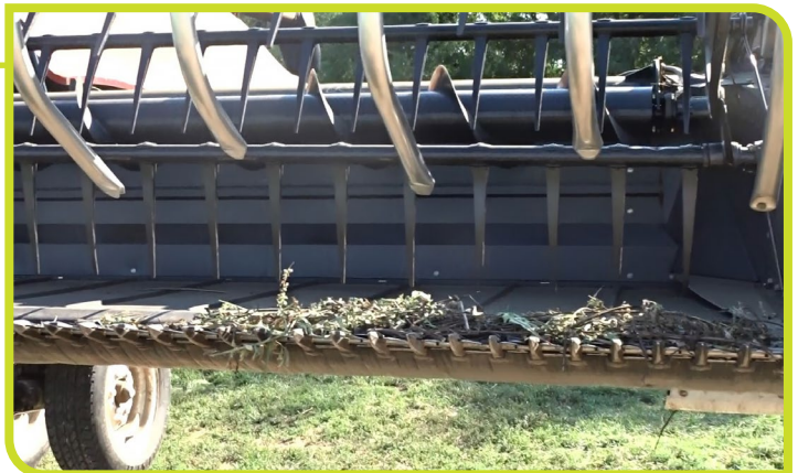
Plant material caught in the sickle sections of the cutting platform. (NDSU photo)
