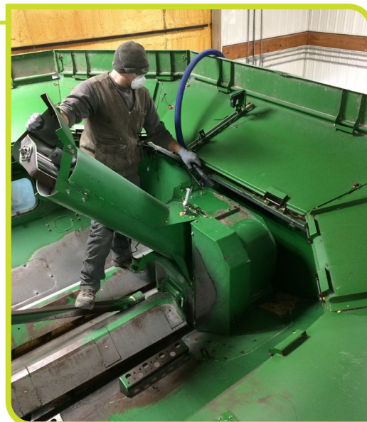
Vacuum the grain tank, starting from top to bottom. (Iowa State University photo)
