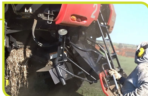
Use compressed air to remove plant material from the chopper. (NDSU photo)
