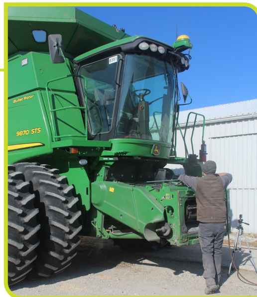
Raise the feeder house and lock it into place. (Iowa State University photo)
