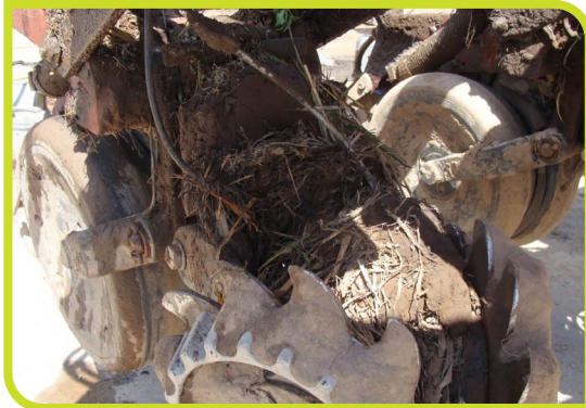
▲ Row cleaners and press wheels are key areas that accumulate unintended biomaterial/soils. (University of Wisconsin-Madison Extension photo)
