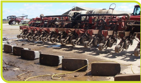
▲ Remove the seed boxes to effectively clean the whole machine. (University of Wisconsin-Madison Extension photo)
