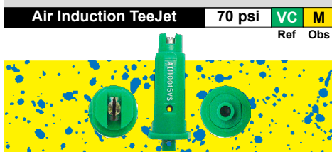
Figure 7. Spray droplet deposits on water-sensitive paper for each of the 15 nozzles in the representative nozzle set at the indicated operating pressure and 8 gpa water volume. Also included are the reference spray qualities (Ref) taken from manufacturer nozzle catalogs and the observed spray qualities (Obs) according to D_{v0.1} , D_{v0.5} and D_{v0.9} values returned by WRK DropletScan™ spray droplet analysis software. Spray qualities are according to ASABE S572.1. NDSU graphic.
