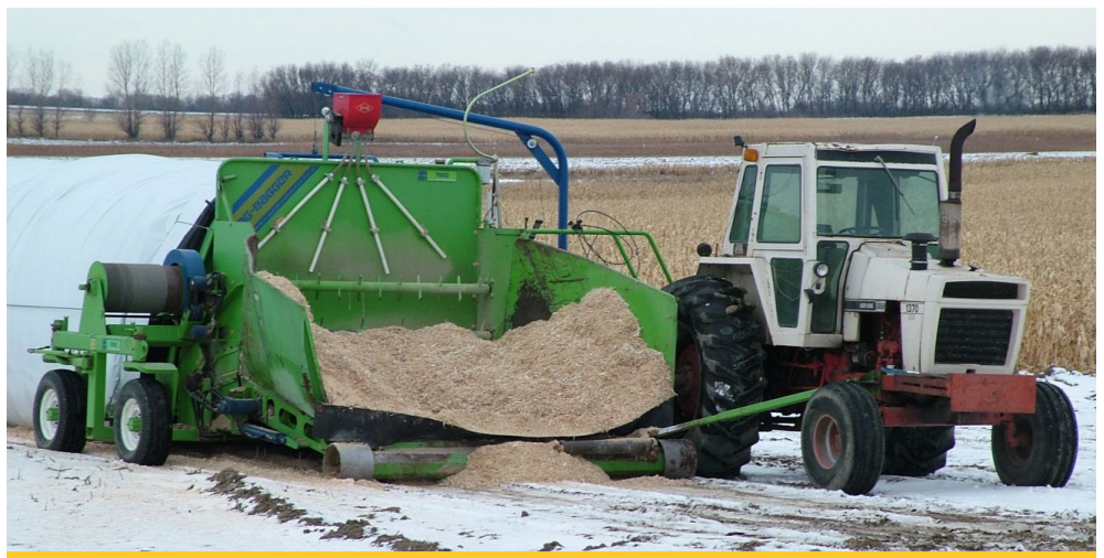
Photo 4. A large-capacity bagger for placing feed ingredients in anaerobic storage. (Greg Lardy, NDSU)
