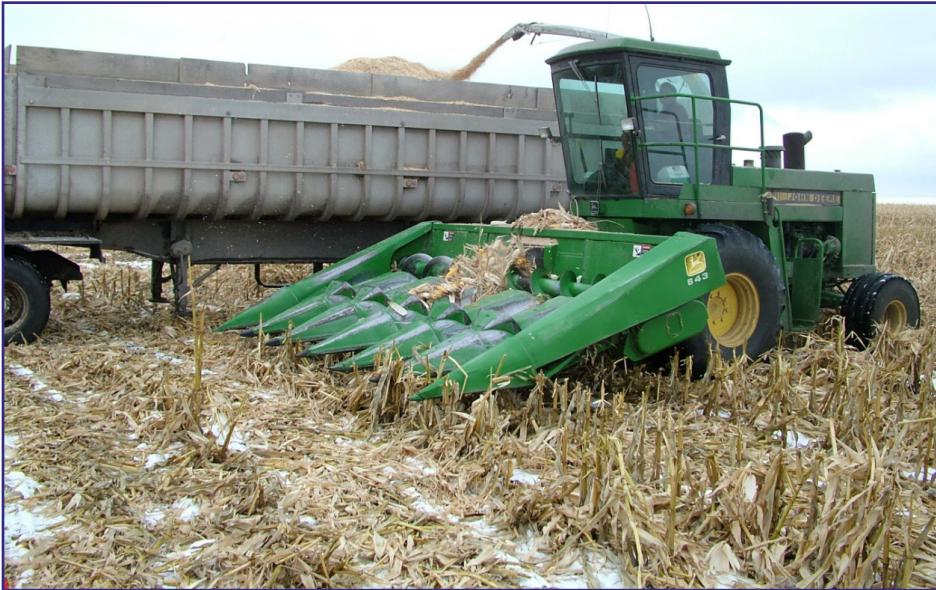
Figure 2. Harvesting snaplage in northeastern North Dakota using a self-propelled forage harvester and a snapper head.
