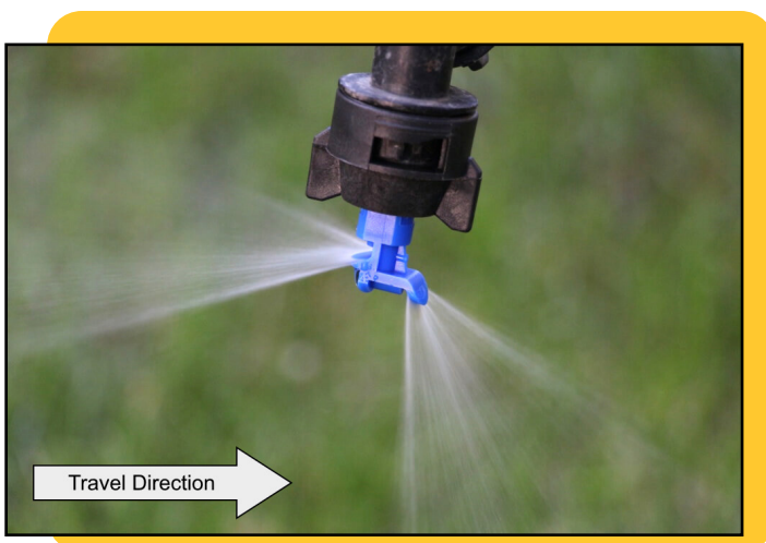
Figure 2. TeeJet AI3070, an asymmetrical twin fan nozzle recommended for FHB suppression.
