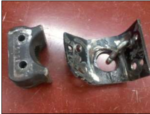
Figure 7: Failed Axle Coupling System from the Bison Pullers Model 1131 Tractor
