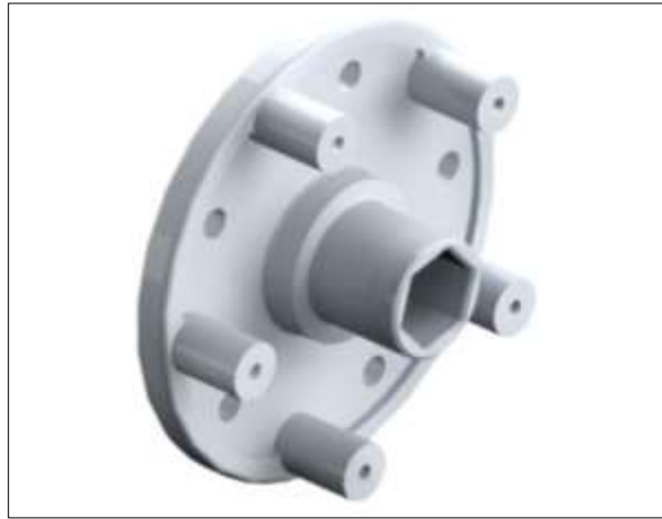
Figure 11: Redesigned Five-Bolt Hub with Hexagonal Bore
