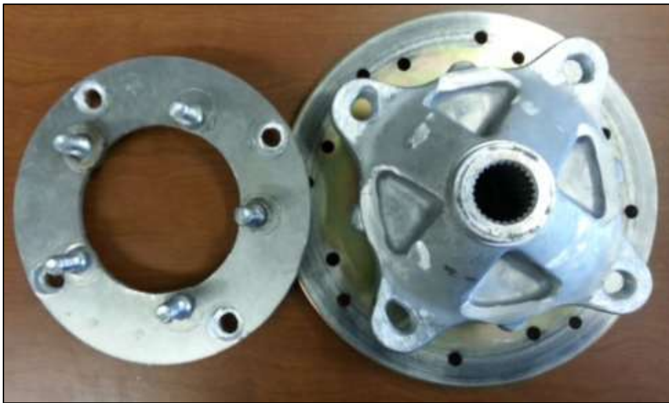
Figure 10: Failed Hub and Hub Adapter used on the Bison Pullers' Model 1231 Tractor
