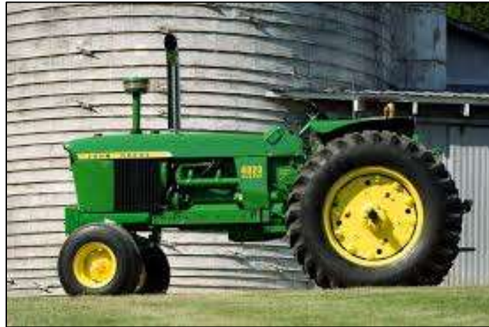
Figure 3: John Deere 4020, which uses the basic Independent Rear-Wheel Drive system. (Swope, 2010)
