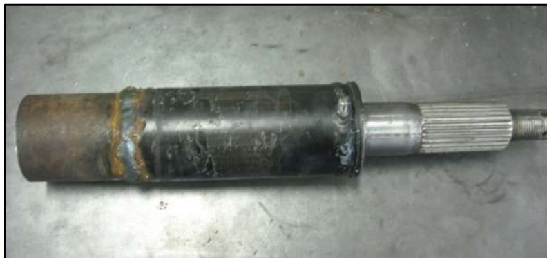
Figure 8: Redesigned Axle Shaft Coupler System used to repair the Model 1131 Tractor
