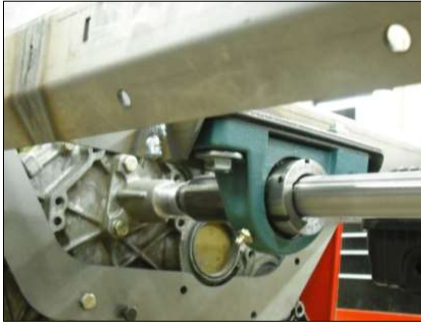
Figure 21: Greased Lubrication Access for Dodge GT 206 Bearings (Baldor Electric Company, 2013)
