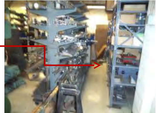
Area 2: Material storage in room; narrow aisle is safety concern
