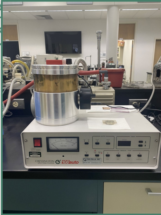
Fig 10: Sputter coater used to coat the thin section in gold (Au)
