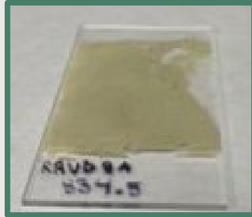
Fig 17: RRVD 8A 534.5' prepared for XRD
