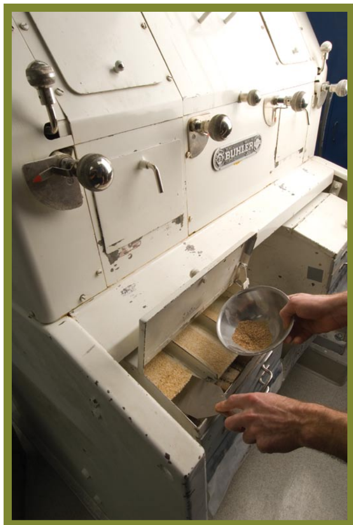
Buhler MLU-202 laboratory mill.
