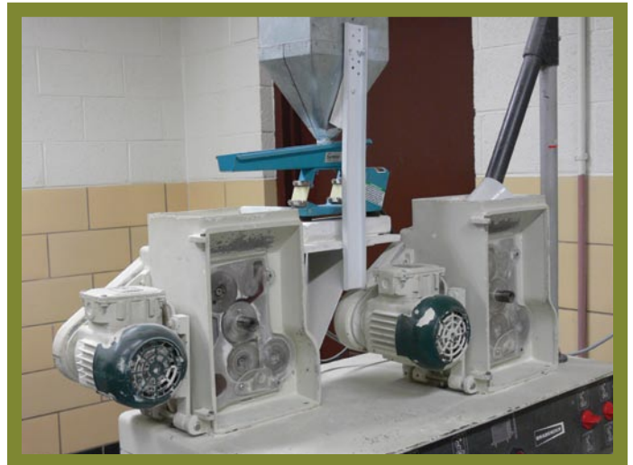
Brabender Qudramat Sr. grinding rolls.
