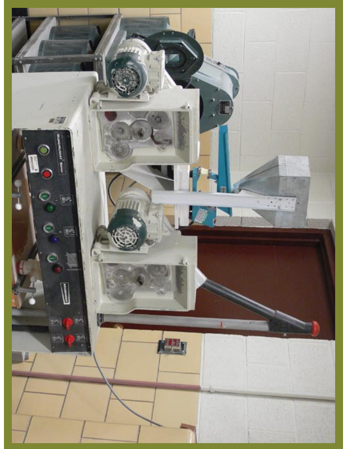
Brabender Qudramat Sr. laboratory mill.
