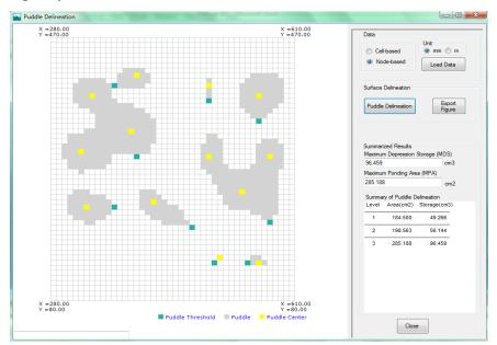
4) <u>Specify the Locations of Points</u>: To manually specify any point in the depression, users can check "Add Point," and then specify any points manually in the depressions by left-
