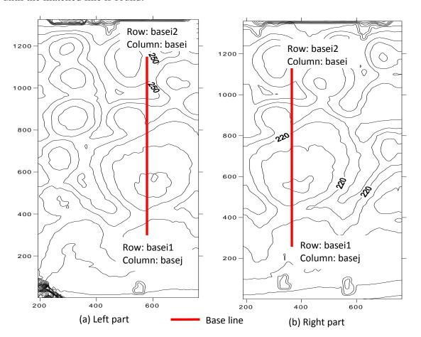
Since the same object in the two files may have different elevations, the total error of the elevations of the matched part will be minimized:
